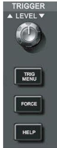
Figura 1-11 Menu do Trigger no Painel Frontal
